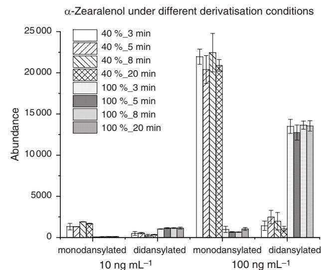
**Fig. 1.** Various derivatisation conditions and LC-MS/MS determined abundances of monodansylated and didansylated products of mycoestrogen  $\alpha$ -zearalenol. Data are shown for two concentrations of the compound ( $10$  and  $100 \text{ ng mL}^{-1}$ ). Four incubation intervals (3, 5, 8, 20 min) and two volumes of derivatisation reagents (40 and 100% of the total volume) were tested.
